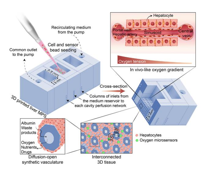
Schematic of the liver MPS hydrogel chip. Cells or spheroids are seeded by pipetting directly into each of the three culture cavities, without or with addition of oxygen sensor beads. The immersed 3D printed chip is perfused in a simple loop between the inlet and outlet, with the surrounding medium functioning as
