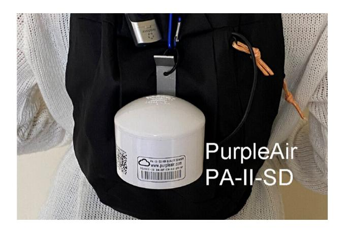
PurpleAir attached to customized backpack and powered by battery pack (inside). The PurpleAir was secured in place with Velcro to minimize agitating fiber particles and to keep the sensor as close as feasibly possible to 'breathing zone' height. When stationary for long periods, the participant was permitted to remove the PurpleAir from the backpack and keep it close-by. Credit: *Social Science & Medicine* (2023). DOI: 10.1016/j.socscimed.2023.116293
