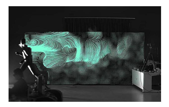
Researchers moved a mannequin equipped with a device that emits aerosol particles to examine the number and movement of the particles. Credit: Takeshi Asai, professor emeritus at the University of Tsukuba
