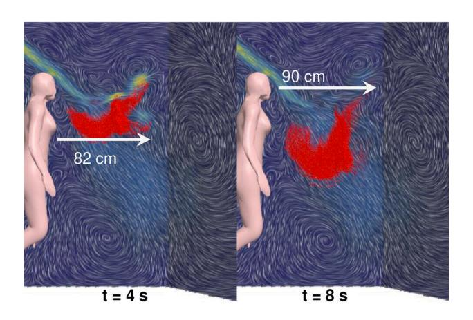
Snapshots of the droplets and flow field at various instances for a volumetric flow rate of 120 m<sup>3</sup>/h (three air changes per hour). Credit: Dimitris Drikakis
