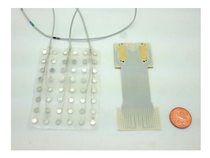
Compared to current speech prosthetics with 128 electrodes (left), Duke engineers have developed a new device that accommodates twice as many sensors in a significantly smaller footprint. Credit: Dan Vahaba/Duke University
