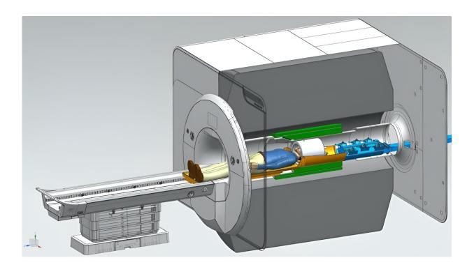
Cross-sectional diagram of the NexGen 7T scanner, showing the new Impulse head-only gradient coil (green) and receiver-transmit coil (white) resting on a movable bed (brown) and connected to an electronic interface (blue) containing nearly a thousand wires (blue) that extend out of the magnet. Credit: Bernhard Gruber, MGH Harvard
