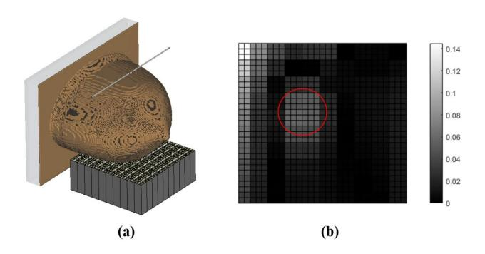
(a) The simulation setup of the ACR Class 2- Scattered Fibroglandular breast phantom (b) the obtained impression, where the red circle indicates the border of the tumor with a radius of 1.5 cm. Credit: *Scientific Reports* (2023). DOI: 10.1038/s41598-023-40494-x
