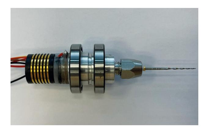
Dental file demonstrator with integrated piezoceramic stack actuator. Credit: Fraunhofer-Gesellschaft
