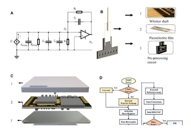
The design of the proposed hardware system for artificial whisker-based sensing, which comprises a whisker-based sensor, signal conditioning circuits, and the embedded control algorithm. A A pre-processing circuit (labeled as 3 in B), a charge amplifier, is designed to achieve impedance matching, as well as the
