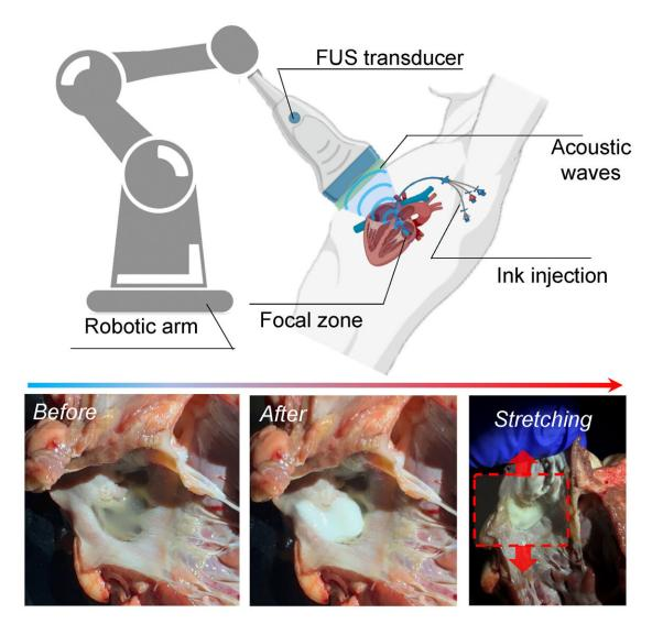
In this example, DAVP is used to close the left atrial appendage (LAA) in a goat heart, which can reduce the risk of forming blood clots inside the heart. The printed construct conforms to the heart wall, and is highly stretchable. DAVP does not need to open the chest for such a heart surgery. Credit: Junjie Yao, Duke University; Shrike Yu Zhang, Harvard Medical School
