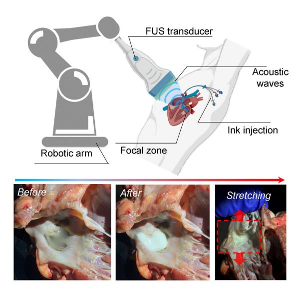
In this example, DAVP is used to close the left atrial appendage (LAA) in a goat heart, which can reduce the risk of forming blood clots inside the heart. The printed construct conforms to the heart wall, and is highly stretchable. DAVP does not need to open the chest for such a heart surgery. Credit: Junjie Yao, Duke University; Shrike Yu Zhang, Harvard Medical School
