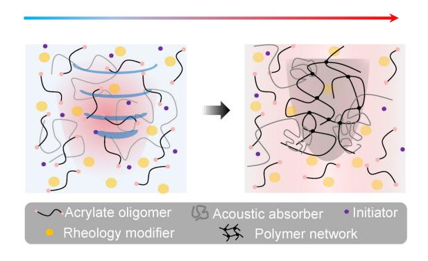
DAVP prints 3D constructs by curing sono-inks with focused ultrasound waves. The sono-thermal effect triggers the decomposition of the sono-inks to form polymer networks at the ultrasound focal zone. Credit: Junjie Yao, Duke University; Shrike Yu Zhang, Harvard Medical School.
