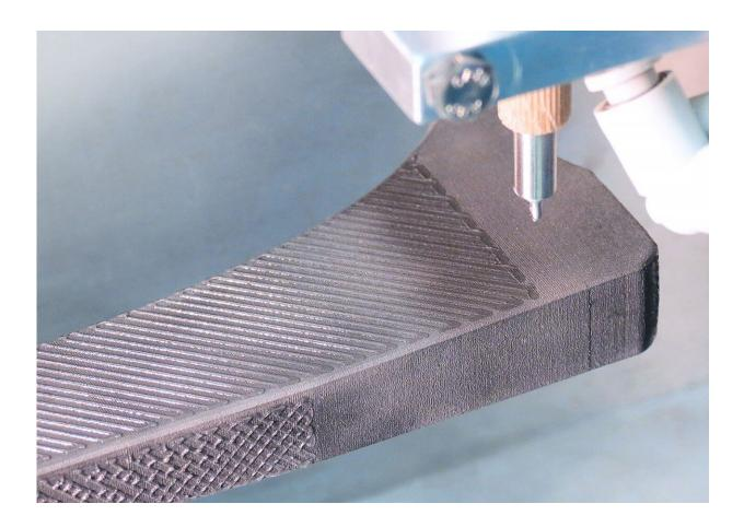
A printer applies the dopamine-based tissue adhesive to the three-dimensional titanium shaft of a hip joint. Credit: Fraunhofer-Gesellschaft
