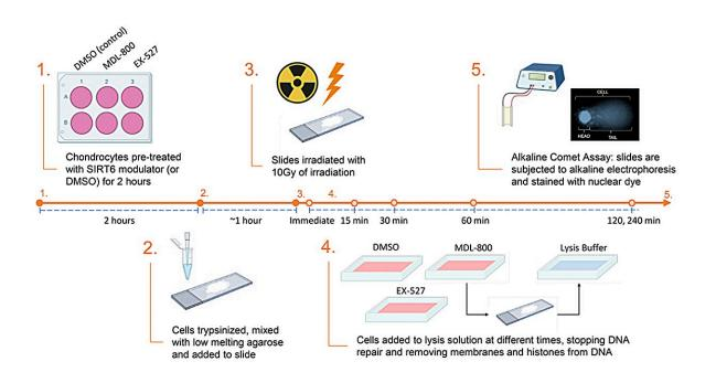
Experimental design for the results shown in Figures 3 and 4. Credit: 2023 Copp et al.
