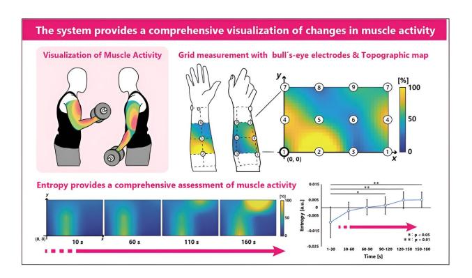
The traditional sEMG approaches are unable to evaluate the activity of multiple muscles at the same time. This is important to study the coordination of muscles in the human body. To overcome this limitation, researchers from Japan have established a novel measurement system and demonstrated its effectiveness. Credit: Ms. Megumi Shimura and Dr. Yoshihiro Shimomura, Chiba University, Japan
