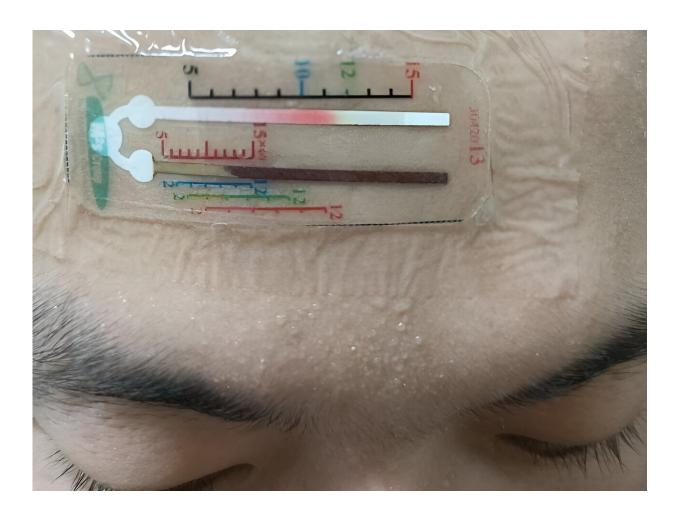
A wearable sensor, developed by Penn State researchers, accurately detects biomarker concentrations in sweat samples. Credit: Larry Cheng
