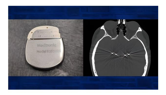
The new device (left) acts like a pacemaker that can adjust the parameters of stimulation automatically. The CT scan (right) shows the placement of four electrodes to deliver the stimulation. Credit: Duke University
