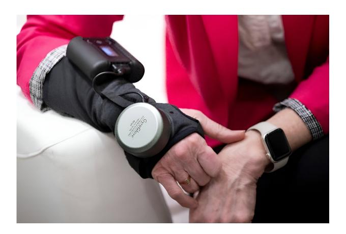
A GyroGlove that counters tremors caused by Parkinson's disease contains inner workings that spin faster than a jet turbine, and its creators at GyroGear are keen to reduce its size in future versions.
