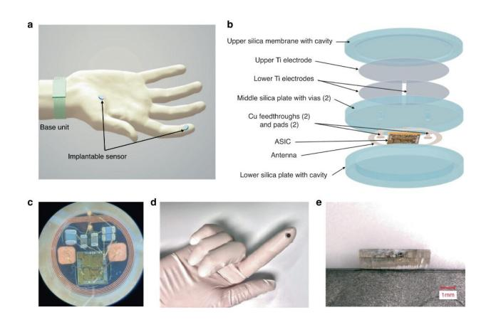
Implantable, wireless, battery-free tactile sensing system. Credit: *Microsystems & Nanoengineering*
