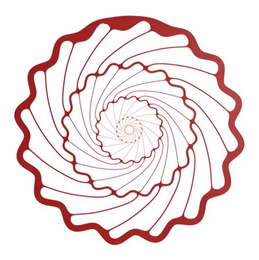
Top view of a Kirigami electrode mesh. Credit: Cui lab and Pasca lab
