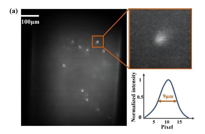
Figure 2 (a) Leukocytes in a channel captured by a miniature fluorescence microscope, with a magnified view of one of the cells and its profile curve. (b) Working process of the particle counting algorithm. Scale bar: 100 μm. Credit: *Opto-Electronic Science* (2023). DOI: 10.29026/oes.2023.230018
