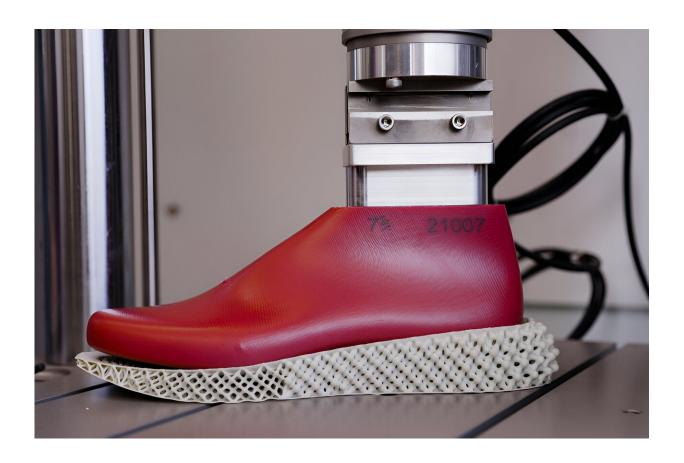
Researchers measure the stiffness of midsole designs using an Instron machine to mimic footsteps. Credit: Melanie Gonick, MIT
