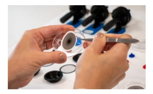
Dust samples are collected on filters for analysis with UQ's Mineral Liberation Analyser. Credit: University of Queensland
