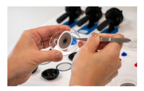
Dust samples are collected on filters for analysis with UQ's Mineral Liberation Analyser. Credit: University of Queensland
