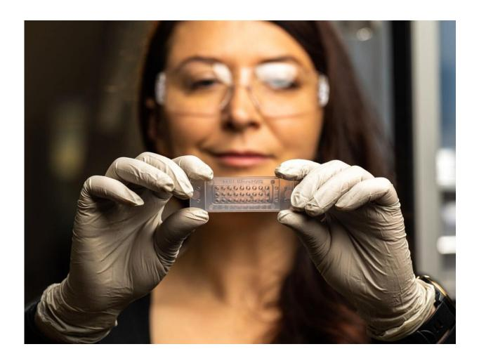
MicroPOTS is a chip-based approach developed by Pacific Northwest National Laboratory that allows sample processing in a microliter droplet to greatly improve the sensitivity of proteomics measurements. Credit: Andrea Starr | Pacific Northwest National Laboratory
