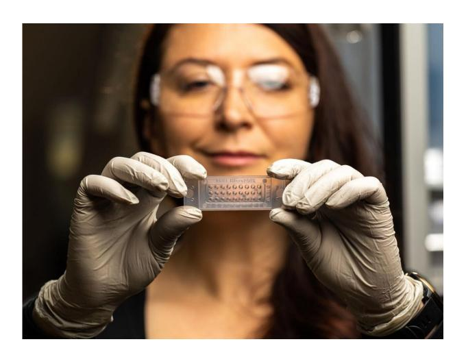
MicroPOTS is a chip-based approach developed by Pacific Northwest National Laboratory that allows sample processing in a microliter droplet to greatly improve the sensitivity of proteomics measurements. Credit: Andrea Starr | Pacific Northwest National Laboratory
