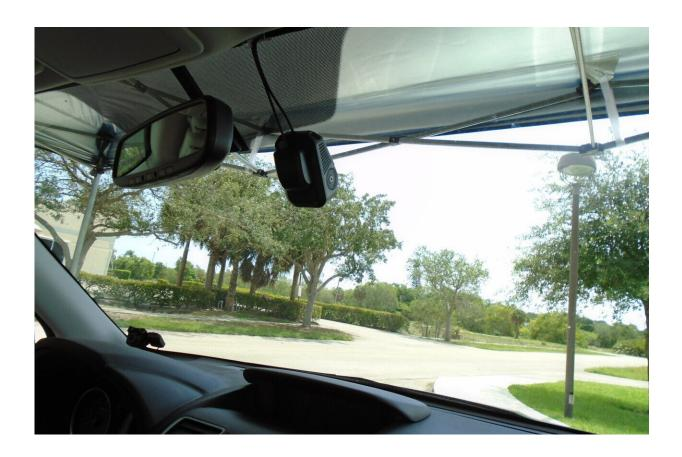
The driver-facing camera is mounted in the left corner of the windshield and is directed to the driver's face to analyze his/her behavior and facial expressions. The forward-facing camera is mounted under the rearview mirror and is used to record events external to the vehicle. Credit: Jinwoo Jang, Ph.D., FAU College of Engineering and Computer Science
