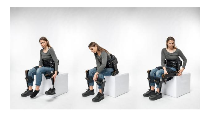
Two features make TWIN unique in the world: it is made of lightweight materials, such as aluminum alloy, and it is composed of modular components, facilitating usability and transportation. Credit: IIT-Istituto Italiano di Tecnologia
