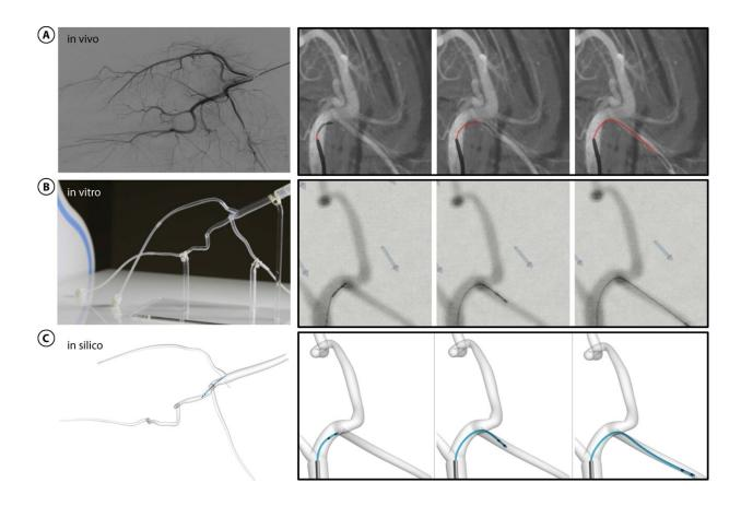
Side-by-side comparison of in vivo, in vitro, and in silico navigation. (A) In vivo navigation. It serves as a ground truth for the simulated navigations. (B) In vitro navigation. (C) In silico navigation. Credit: ETH Zurich
