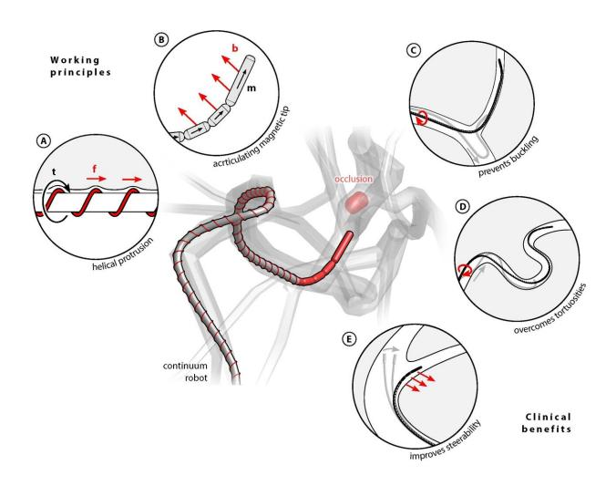
Helical mCR with articulated magnetic tip. (A) The helical protrusion on the outer surface of the continuum robot, upon rotation, pushes the robot tip forward. (B) The segmented articulating magnetic tip increases the magnetic volume and decreases bending stiffness for improved steerability. (C) The helical robot prevents buckling and (D) overcomes tortuous vessels. (E) The
