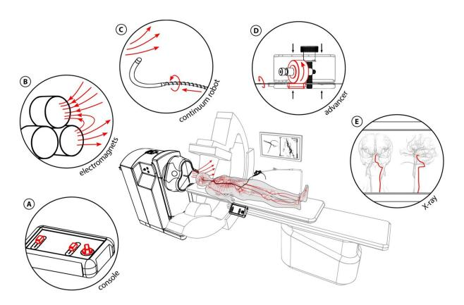
Helical mCR with articulated magnetic tip. (A) The helical protrusion on the outer surface of the continuum robot, upon rotation, pushes the robot tip forward. (B) The segmented articulating magnetic tip increases the magnetic volume and decreases bending stiffness for improved steerability. (C) The helical robot prevents buckling and (D) overcomes tortuous vessels. (E) The articulating tip allows for large tip deflections. Credit: ETH Zurich
