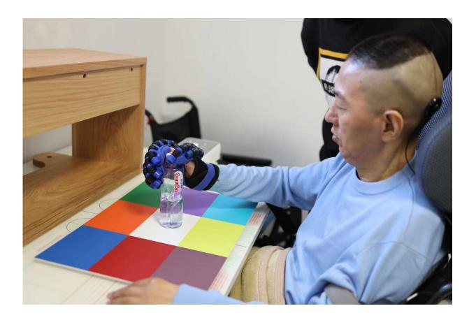
The patient grasps a bottle using the NEO wireless BCI system and a prosthetic hand. Electrodes were implanted over his primary sensory and motor cortex (S1 and M1) to collect ECoG signals above the dura matter, while he attempted to grasp the bottle. Credit: Tsinghua University
