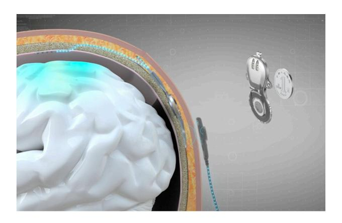
Wireless minimally invasive BCI – NEO system. Epi-dural electrode array are implanted in the skull above the functional localized area, collecting local field potentials, which makes neural tissues intact. The chips buried in the skull enable wireless power induction and signal transmission, which makes a no-battery implantation. Credit: Tsinghua University
