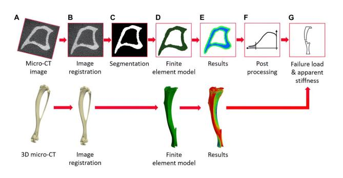
Flowchart illustrating the main steps of the pipeline to create the micro-FE models from the micro-CT images and to evaluate the apparent mechanical properties (from (A–G)) micro-CT acquisition, image registration, image segmentation (binarization), creation of the micro-FE models, results generation, post-processing of the local strains, calculation of failure load and apparent stiffness. Credit: *Frontiers in Bioengineering and Biotechnology* (2024). DOI: 10.3389/fbioe.2024.1335955
