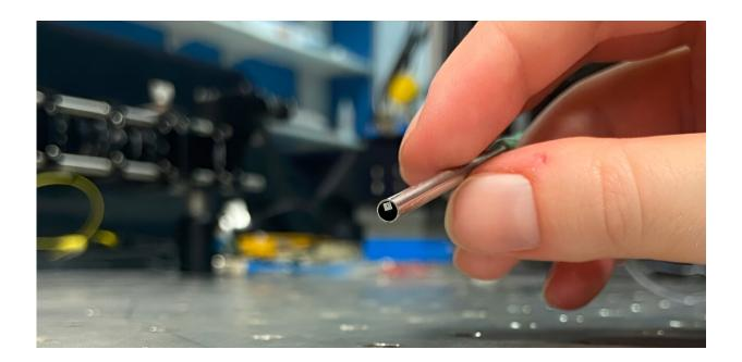
The ultraminiature SFDI system is designed to be incorporated into colonoscopes. By leveraging the phenomenon of light interference, the endoscopic system can reveal information about the optical properties of tissue under investigation. In this photo, Dr. Jane Crowley holds a prototype device, in which the 3-mm diameter fiber tip encases the ultraminiature camera. Credit: J. Crowley.
