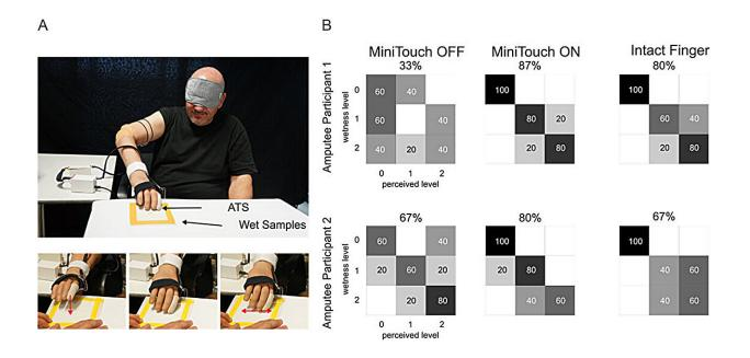
Active scanning of wet samples with a prosthetic hand. Credit: *Advanced Intelligent Systems* (2024). DOI: 10.1002/aisy.202300512
