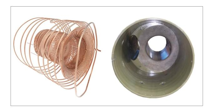
The coils that generate the magnetic field (left) and a visualization of the entire scanner (right). Credit: ETH Zurich
