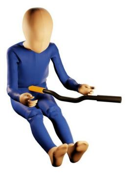
Simulation of the impact on the end of a handlebar. Credit: VSI-TU Graz
