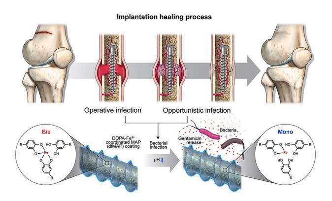
Schematic depicting a functional implant coating material designed to promptly release antibiotics in reaction to alterations in the body's environment induced by bacterial infection. Credit: POSTECH
