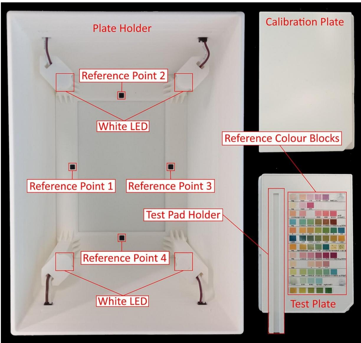
The prototype device includes a plate holder with four white LEDs and four reference points, a calibration plate and a test plate with reference color blocks and a test pad holder. Credit: *Methods* (2024). DOI: 10.1016/j.ymeth.2024.02.002
