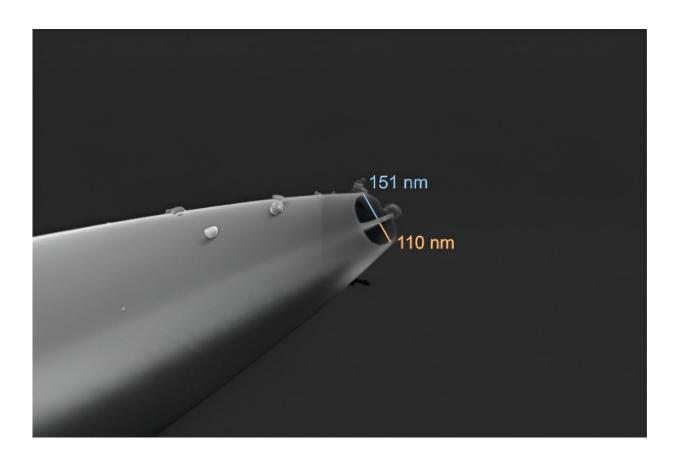
Electron microscopy image of a nanopipette (image acquired using a scanning electron microscope (SEM)). Credit: Dr. Alexander Kulak
