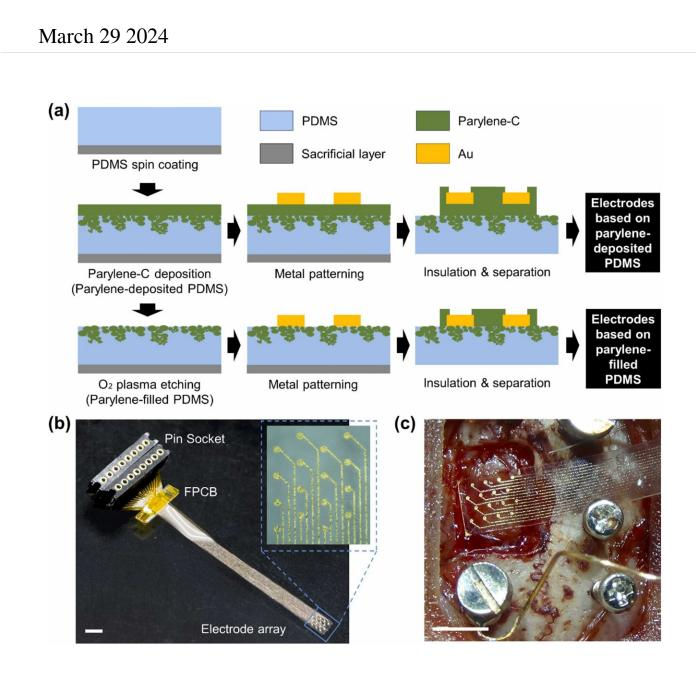
ECoG electrode array based on PDMS-based substrates treated in two different
