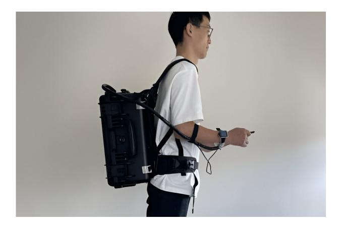
The system consists of a watch with an imaging interface, a handheld computer and a backpack housing the laser and power supply. It is designed to allow imaging while the wearer moves around freely. Credit: Lei Xi, Southern University of Science and Technology
