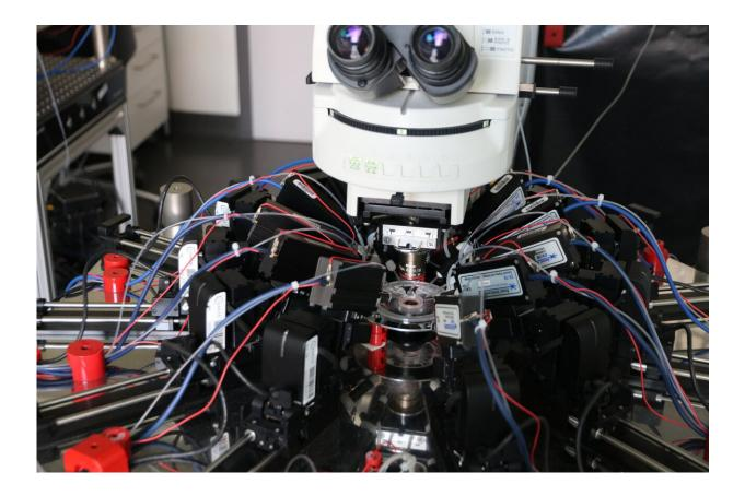
Experimental setup for multi-patch experiments that record the activity of up to ten neurons. Credit: Charité | Yangfan Peng
