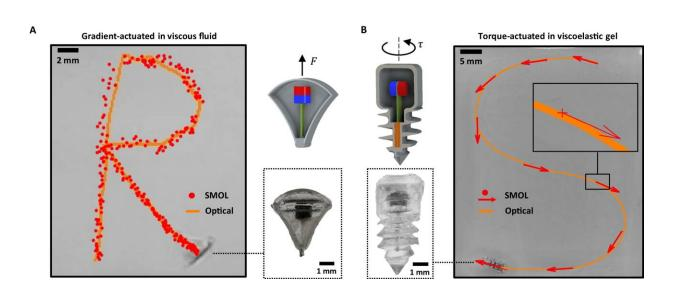
Integration of SMOL and actuation in millirobots. Credit: *npj Robotics* (2024). DOI: 10.1038/s44182-024-00008-x
