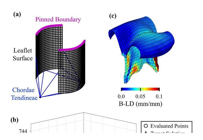
a Schematic of the simplified model for two leaflets in contact. b Element-wise bidirectional local distance (B-LD) errors for the optimal BO solution normalized by the characteristic length (4.03 mm). c Mean Gaussian process surface from the BO procedure. Credit: *Annals of Biomedical Engineering* (2023). DOI: 10.1007/s10439-023-03408-6
