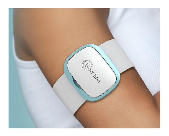
The Biovotion Everion wearable device we used to collect physiological and behavioral sensor data over the day. Image: Infinity Design. Credit: *npj Digital Medicine* (2024). DOI: 10.1038/s41746-024-01025-8
