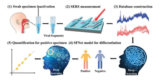
Schematic illustration of direct quantitative detection from HNS specimens using SERS and DLAs. Credit: *Advanced Materials Interfaces* (2024). DOI: 10.1002/admi.202400013
