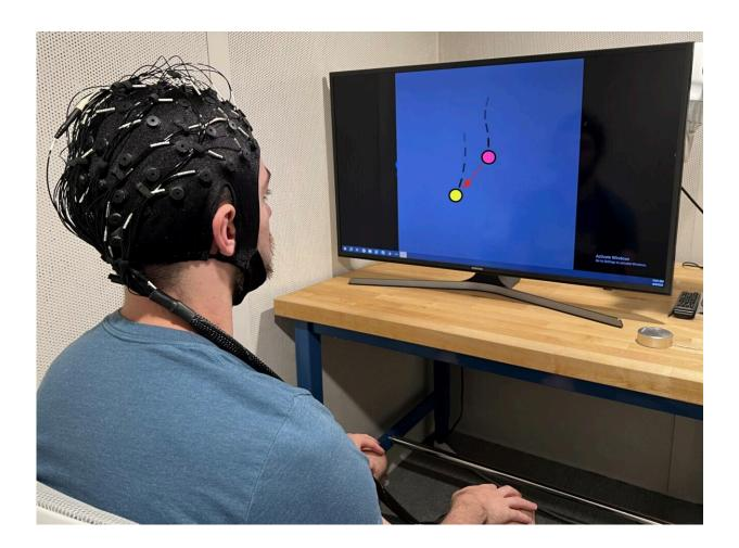
A BCI setup, where the user is interacting with a computer with their intention recorded and decoded from EEG. Credit: Forenzo et al
