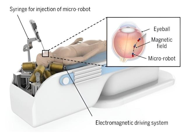
An electromagnetic driving system manipulates a micro-robot within the patient's posterior eye. Credit: Scientists from the School of Mechanical Engineering, Tianjin University.
