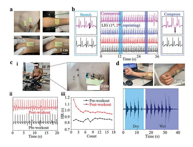
Biopotential measurements by the LIG@PI/PDMS/PEIE-based adhesive patch. Credit: *Advanced Materials* (2024). DOI: 10.1002/adma.202400236
