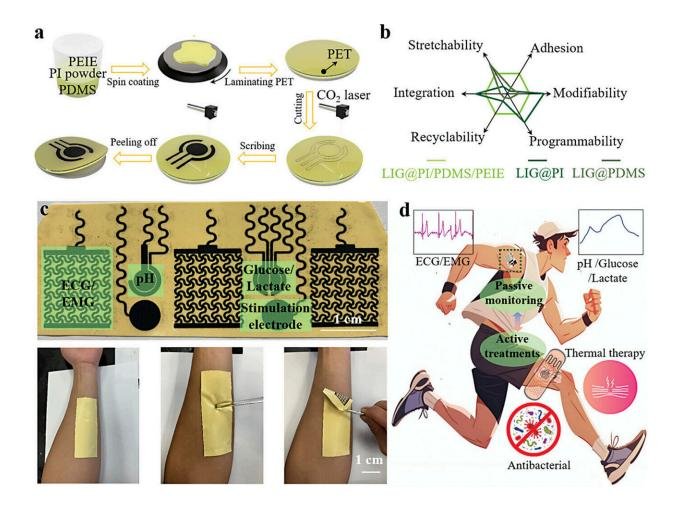
LIG@PI/PDMS/PEIE-based multifunctional, recyclable, and adhesive device patch. Credit: *Advanced Materials* (2024). DOI: 10.1002/adma.202400236
