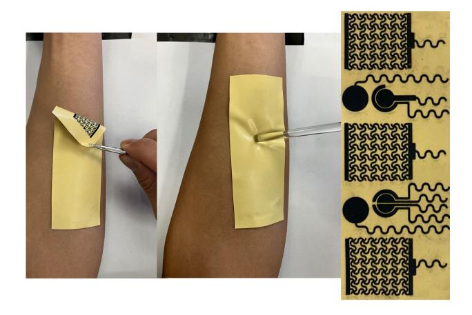
Penn State researchers recently developed an adhesive sensing device that seamlessly attaches to human skin to detect and monitor the wearer's health. The writable sensors can be removed with tape, allowing new sensors to be patterned onto the device. Credit: Jia Zhu/Penn State
