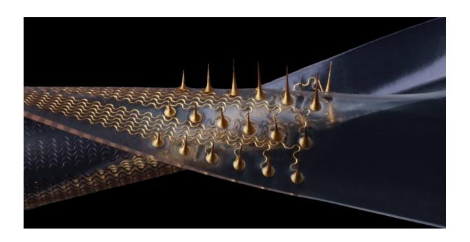
Stretchable microneedle electrode arrays. Credit: Zhao Research Group
