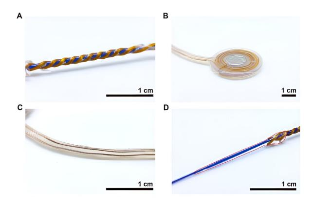
(A-D) Photographs of the components of the strain sensing system. A) Capacitive fiber strain sensor. B) Double-layered inductive coil. C) Transmission lines. D) Conical needle structure. Credit: *ACS Nano* (2024). DOI: 10.1021/acsnano.4c00396
