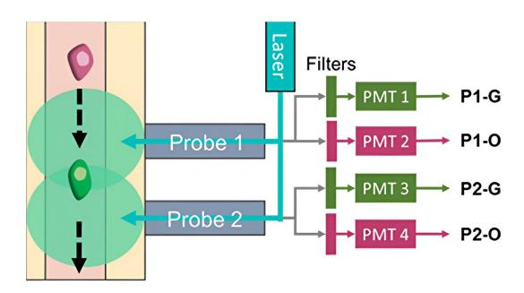
DiFC detects cancer cells expressing fluorescent proteins when the cells are excited by laser light as they move through a blood vessel. Fluorescent light is collected by the DiFC detection fibers and split between two detector arms (filters and photomultiplier tubes) for each fluorophore. Credit: Williams et al., doi 10.1117/1.JBO.29.6.065003.
