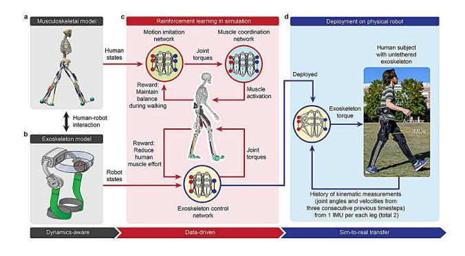
Researchers developed a full-body musculoskeletal human model consisting of 208 muscles (upper left), as well as a custom hip exoskeleton (lower left), then leveraged artificial intelligence to simulate multiple activities (center) before deploying the learned controller on human subjects. Credit: *Nature*, Luo et al.
