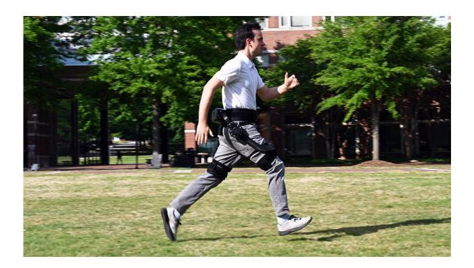
Researchers at North Carolina State University have demonstrated a new method that leverages artificial intelligence and computer simulations to train robotic exoskeletons to autonomously help users save energy while walking, running and climbing stairs. Credit: Hao Su, NC State University
