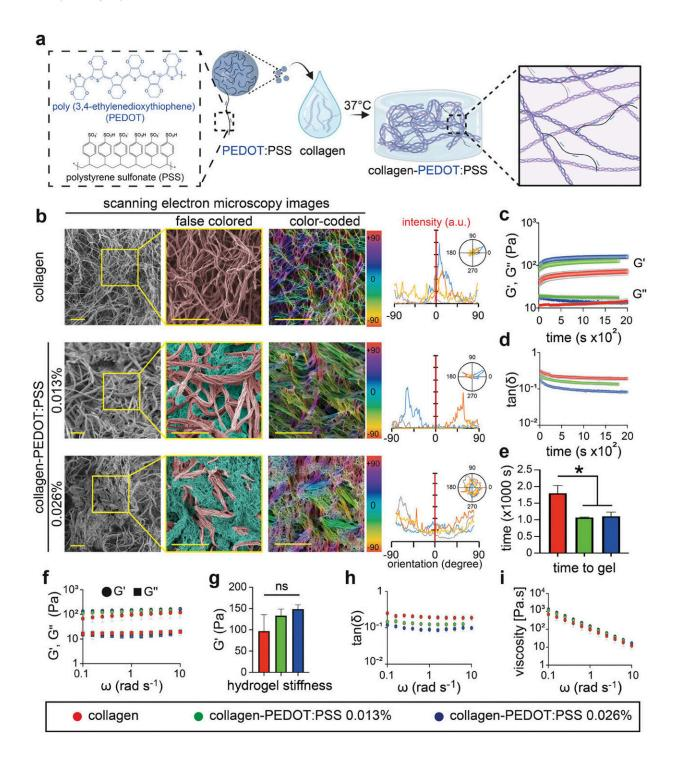
Hydrogel formation and characterization. a) Schematic illustration of hydrogel formation. b) Representative scanning electron microscopy (SEM) images of critical point dried hydrogels and their magnified false-colored regions of interest (ROIs) together with color-coded images and quantified orientation distribution of fibers in each composition. c–e) Characterization of gel
