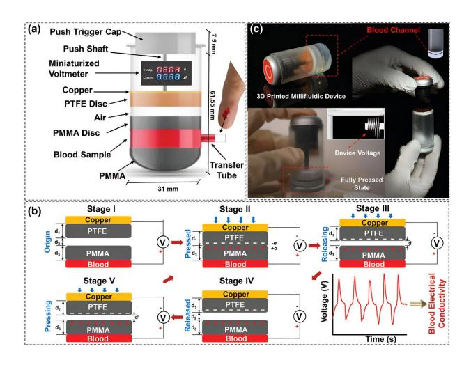
Vision of the proposed research for developing a self-powered, millifluidic labon-a-chip device to determine blood conductivity. Credit: *Advanced Materials* (2024). DOI: 10.1002/adma.202403568
