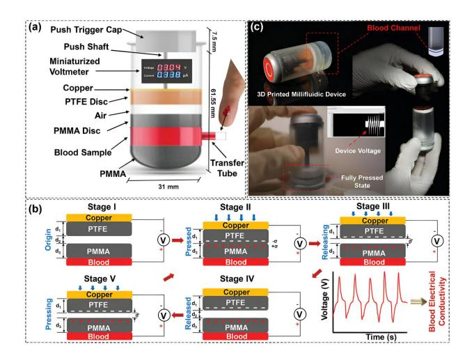
Vision of the proposed research for developing a self-powered, millifluidic labon-a-chip device to determine blood conductivity. Credit: *Advanced Materials* (2024). DOI: 10.1002/adma.202403568
